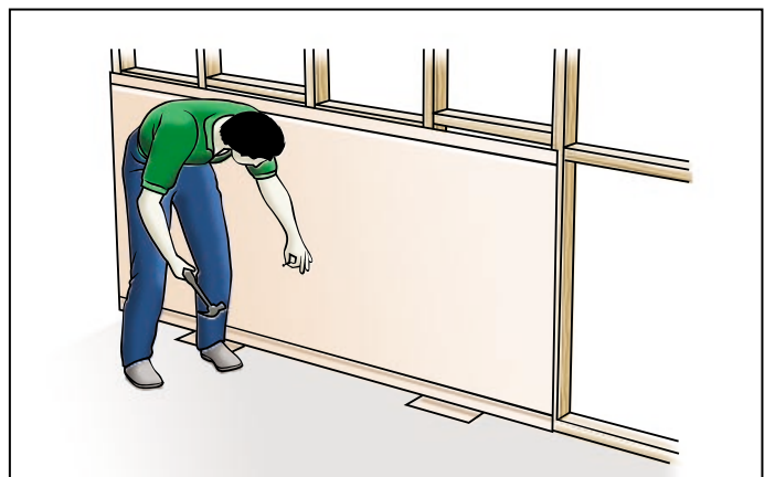
FIGURE 4 FIXING FIRST SHEET
