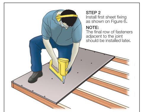
FIGURE 5 FIXING 1ST PANEL
